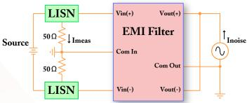
Figure C: Common-Mode Current Attenuation, Imeas / Inoise
