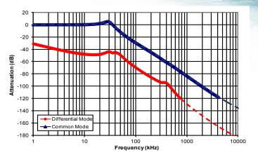
Figure A: Simulation of calculated common-mode and differential-mode current attenuation. The plots show the ratio of the measured current in a  $50\Omega$  LISN sensing port connected to pins 1-6 to the noise current injected into pins 7-12 as shown in Figures B & C.
